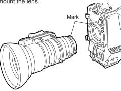
3 Lower the lens clamping lever and clamp the lens.
